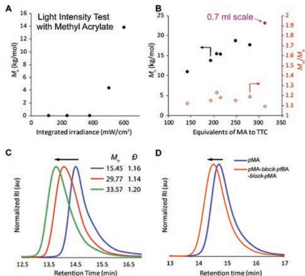
**Fig. 3** (A) Molecular weight dependence on light intensity. (B) Molecular weight and dispersity changes with MA:TTC ratio. (C) GPC traces of chain extension from precipitated pMA to form pseudoblocks. (D) GPC traces of block copolymer synthesis.
