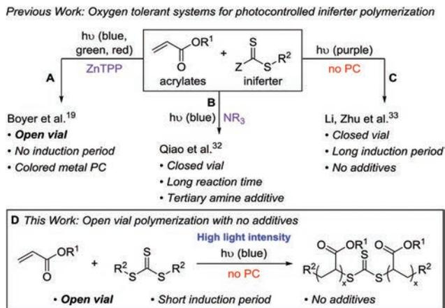
**Fig. 1** Progression of oxygen tolerant CRP using visible light and thiocarbonylthio iniferters: (A) Photocatalyst-mediated CRP in a completely open vial using a metal catalyst. (B) Tertiary amines as sacrificial reductants in photocatalyst-free CRP. (C) Additive-free CRP in a closed vial. (D) Additive-free, open vial CRP utilizing high light intensity.
