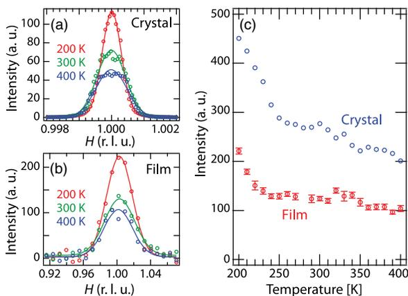
FIG. 4. The scattered intensity of the resonant reflection  $(1\ 0\ 0)$  at various temperatures for (a) a typical film and (b) a bulk crystal. The solid lines are fits to Gaussian profiles. (c) The temperature dependence of the scattered intensity of the resonant reflection  $(1\ 0\ 0)$  for a typical film and bulk crystal.
